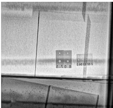
Heavy wall pipe showing sensitivity
