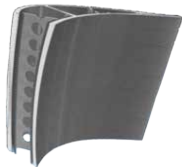
CT Reconstruction of IGT Vane
